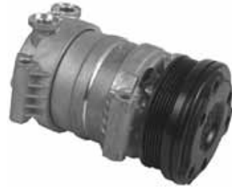
HT-6 6 Cylinder Axial Compressor 12.6 cu. in
