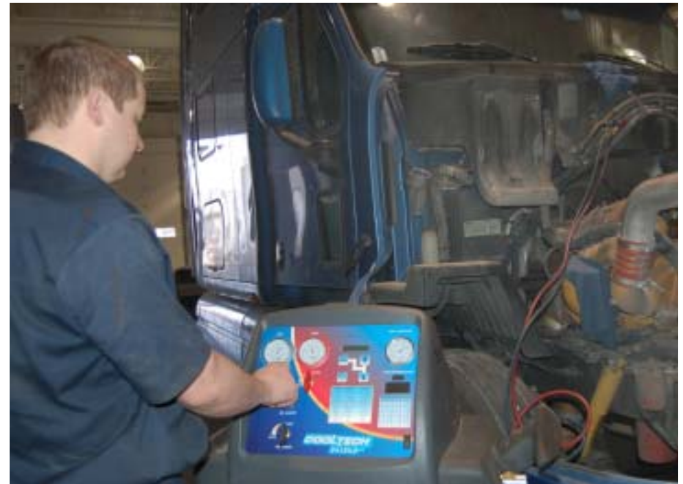
Testing the Freon levels and AC compressor operation.
