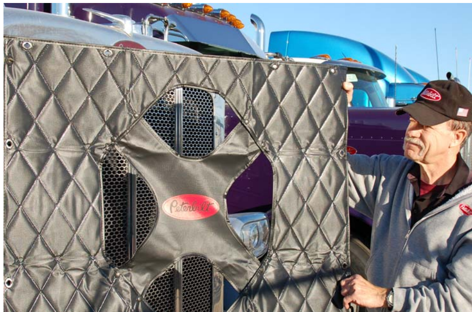
A winter front lets air in, but keeps snow and debris out. Choose certified TRP winter fronts designed to work well with your truck's emissions-control system.
