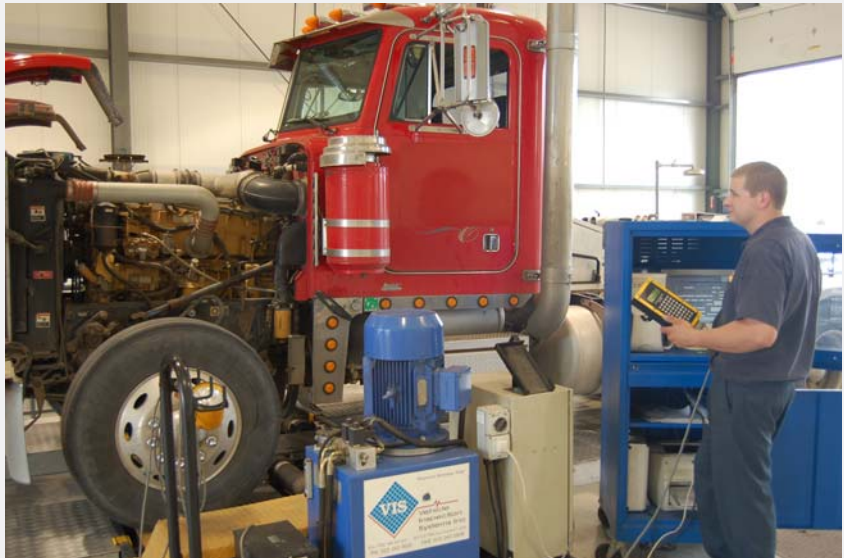
Vis-Check undercarriage diagnostic machine tests for faults
